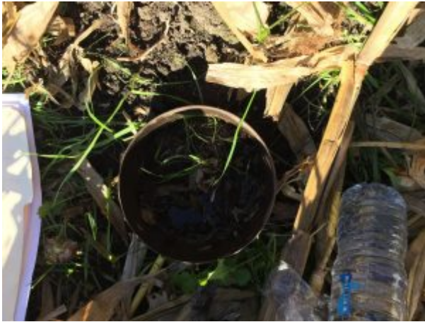
Photo: Infiltration test being completed in corn residue.
